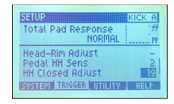
For aD-H12 or aD-H14 pad models: HH Closed Adjust range is -20 to +19
